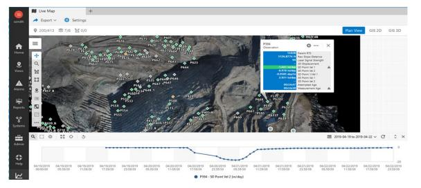
Alarms automatically emailed 24/7 – if radar or prisms trigger alarms, an email is immediately sent to Dispatch, Operations and Mine Engineering
