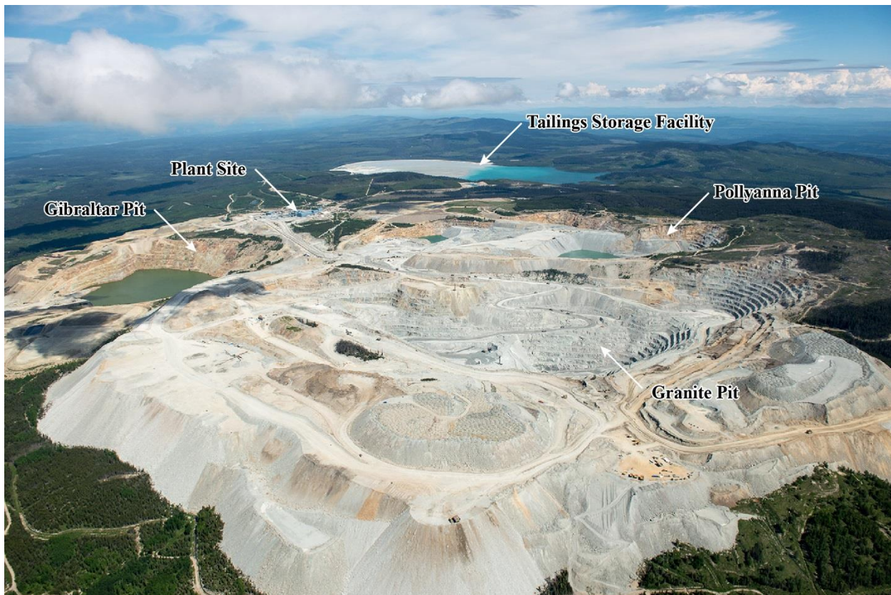
Figure 1-1: Mine Site Configuration
